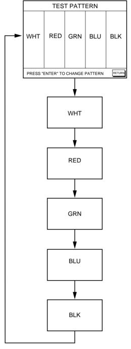
Figure 13-6 Display test pattern
